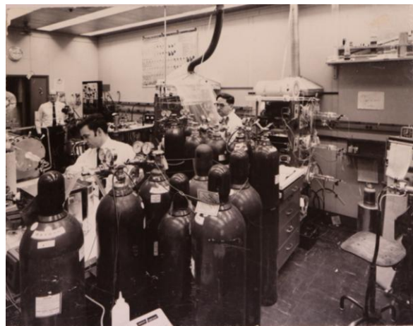
Figure 1: Dale Brown’s “Old Lab Setup” to do research and development for silicon MOSFETs. Left to right: Dale Brown by the door, Richard Connery and George Charney. All the equipment was made in the research lab’s machine and glass shops. The silicon wafers were about one inch in diameter at this time (1964).
